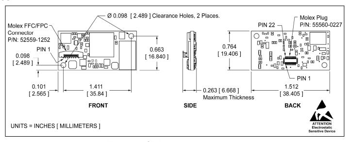
Figure 12. USB Decode Board Dimensions
